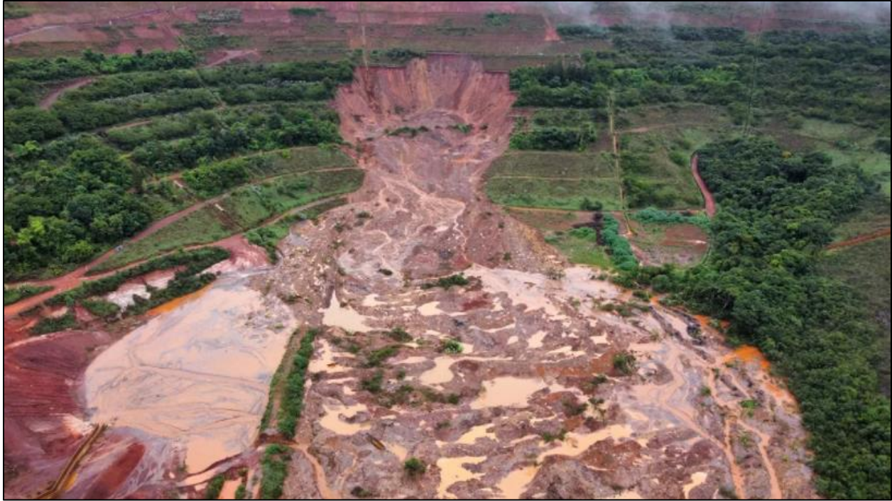
Figure 2. A 48-meter-high filtered tailings storage facility collapsed at the Pau Branco iron-ore mine in Brazil on January 8, 2022. Photo from Angelo (2022).
