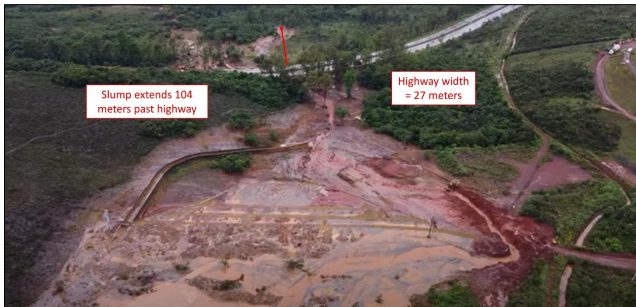
Figure 4a. Based on the highway width of 27 meters, the slump at the filtered tailings storage facility at the Pau Branco mine in Brazil on January 8, 2022 (see Fig. 3), extended for 104 meters past Highway BR-40. Highway width was measured from Google Earth image from June 29, 2022 (see Fig. 4b). Still image at 0:38 of drone video (Observatório da Mineração [Mining Observatory], 2022).
